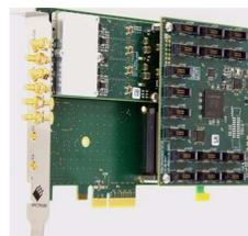
Independent of the number of boards there is no phase delay between all channels. The Star-Hub distributes trigger and clock information between all boards. As a result all connected boards are running with the same clock and the same trigger. All trigger sources can be combined with OR/AND allowing all channels of all cards to be trigger source at the same time.
